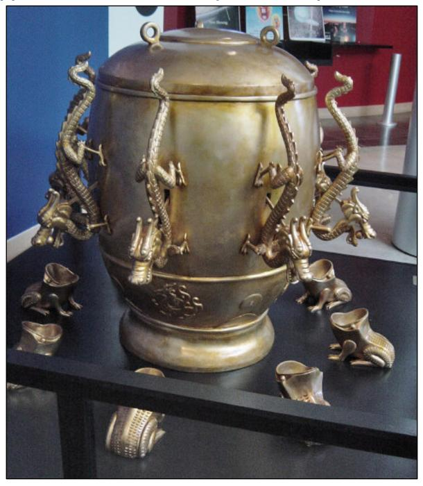
Zhang Heng's seismoscope from 1<sup>st</sup> century BC. A heavy pendulum inside was set swinging and when an earthquake happened it would push a little ball down a ramp, which was used to indicate the direction of the earthquake with mild accuracy.
