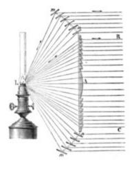
How a spherical Fresnel lens collimates light
