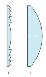
1: Cross section of a spherical Fresnel lens
