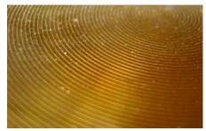
Close-up view of a flat Fresnel lens shows concentric circles on the surface
