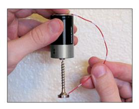
"DIY simple homopolar motor made with a drywall screw, a battery cell, a wire, and a disk magnet. The magnet is on top of the screw head. The screw and magnet make contact with the bottom of the battery cell and are held together by the magnet's attraction. The screw and magnet spin, with the screw tip acting as a bearing."
