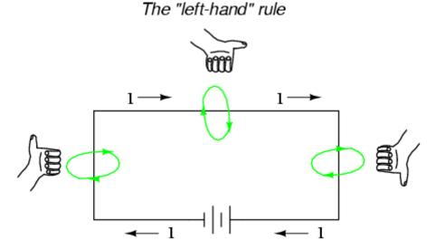
"The magnetic field encircles this straight piece of current-carrying wire, the magnetic flux lines having no definite "north" or "south' poles."
