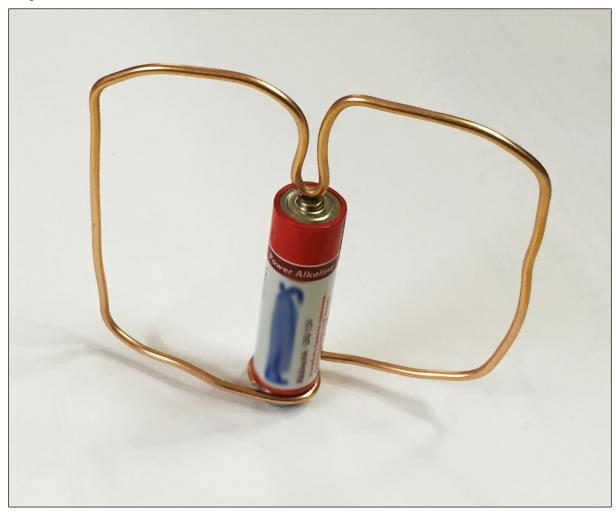
Another simple homopolar motor based off the 'tiny dancer'. Note the wire wraps around the neodymium super magnets very gently, and not around the battery. They must also go in an anticlockwise (from above) direction to maximise push.
